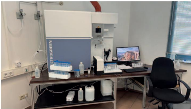
ICP analyzer, used for analyses of, among other things, glass and molten salts be carried out. © ReViSalt GmbH
