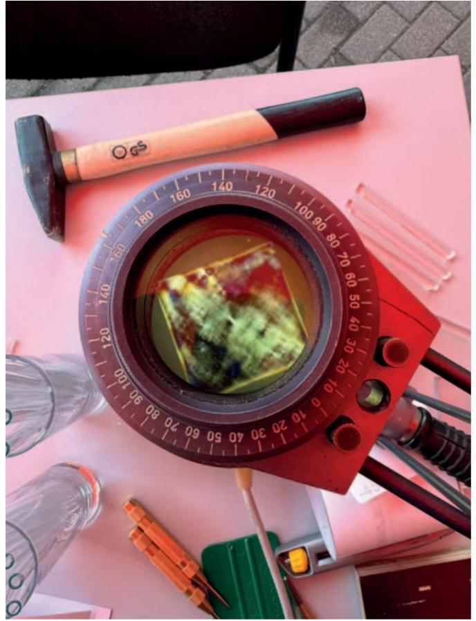
Tempered glass (left); a polariscope can be used to visualize stresses in the glass. © ReViSalt GmbH
