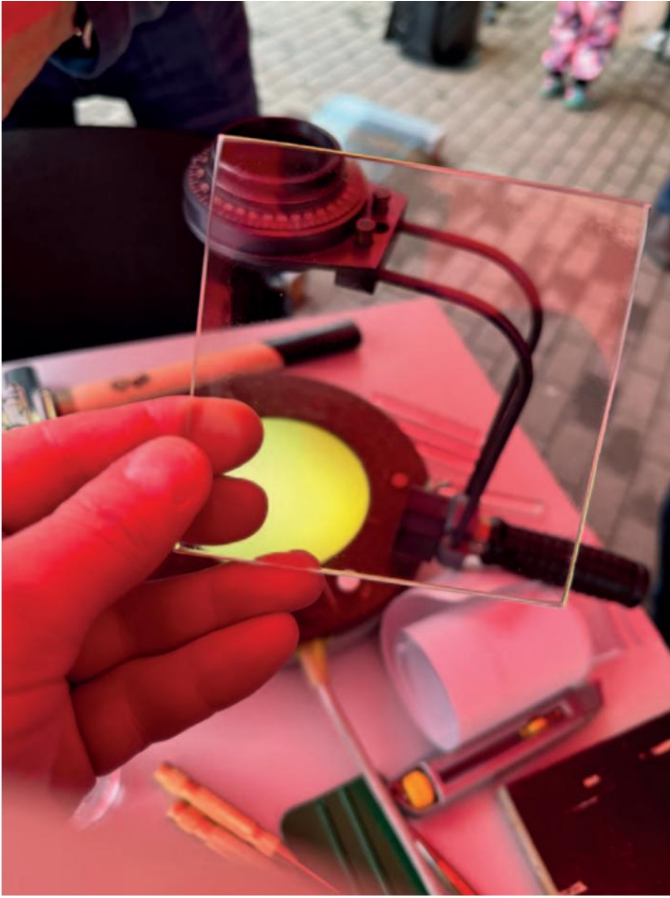
Tempered glass (left); a polariscope can be used to visualize stresses in the glass. © ReViSalt GmbH
